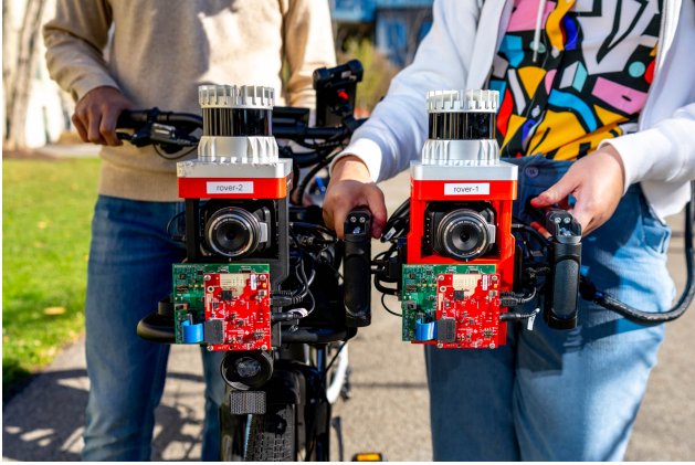
Figure 3. Our data collection rig in its handheld (right) and bike-mounted (left) configurations; see App. A for additional images.
