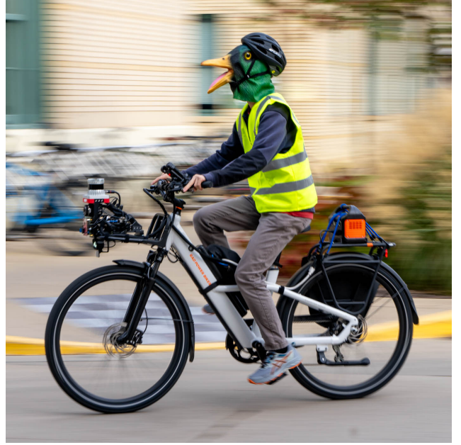
Figure 10. Our data collection system, red-rover , in its bike-mounted configuration. The sensors are mounted to a front rack, while the support electronics are mounted in the center frame and the battery at the rear for balance and stability.
