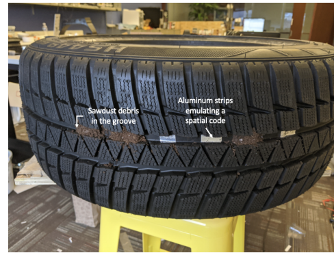
Figure 3: Demonstration of Osprey’s effectiveness in measuring tire wear in the presence of debris using metallic codes.
