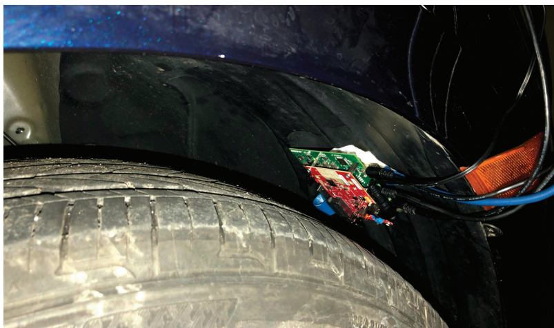
FIGURE 6. Osprey was evaluated in the wild on a passenger car. Osprey's hardware is shown to be mounted on a 2019 Honda Odyssey.
