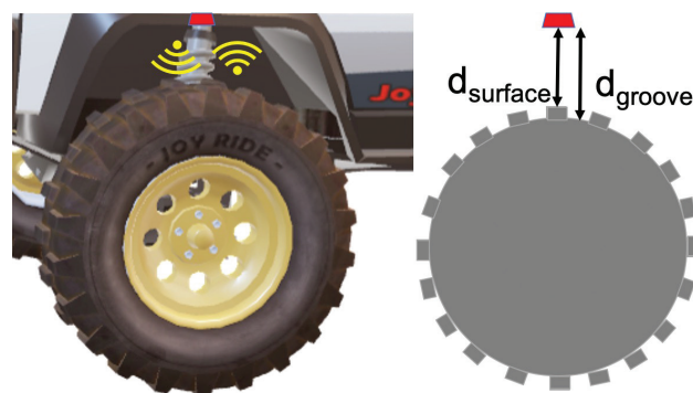
FIGURE 2. Osprey mounts automotive mmWave radar in the tire well, observes reflections from the tire surface and estimates tread depth.
