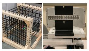
Figure 15: We stress test Platypus in severe multipath conditions by putting the tag in a rebar cage and a in front of a corner reflector.
