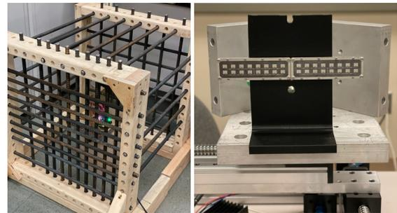
Figure 15: We stress test Platypus in severe multipath conditions by putting the tag in a rebar cage and a in front of a corner reflector.
