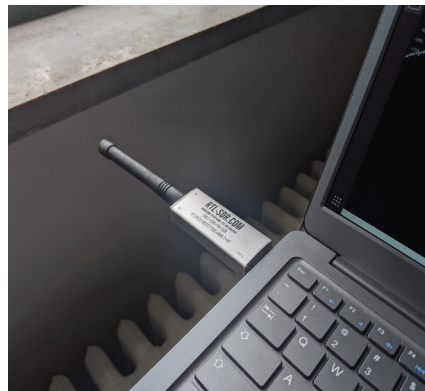
FIGURE 3. Left: Quasar uses tiny RTL SDR receivers with Laird Tuf Duck Antennas, which can be deployed anywhere. Right: Quasar was evaluated on a city scale testbed consisting of both urban and suburban indoor and outdoor structures; red dots indicating locations where low-cost receivers were deployed.
