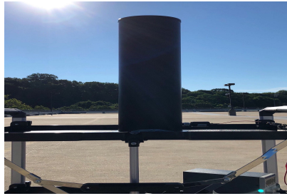
Figure 11: Ground truth antenna installed on rooftop
